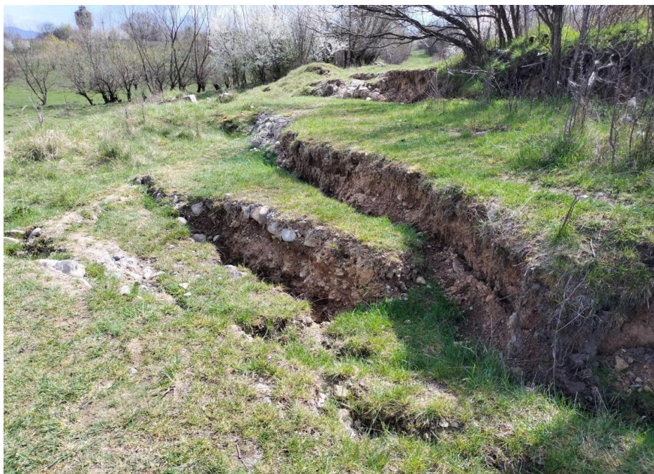
Figure 3 D. Karst-suffusion sinkholes in the mine № 9 eastern flank. General view (Photo 2020-03-17)
