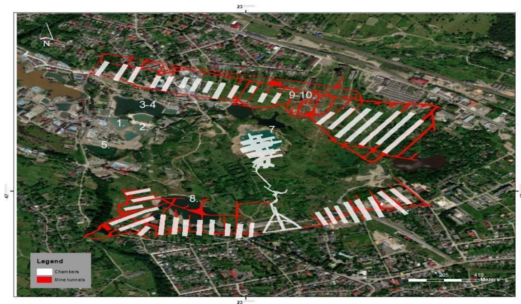
View of today's abandoned mines (white numbering) with the mining chambers and mine openings as potentially and really threatening underground spaces against water ( Geogold Ltd )
